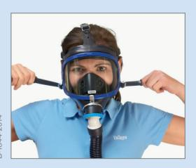
Tighten straps until the mask fits snug and secure. First tighten both neck straps, then both temple straps and tighten front strap if necessary.
