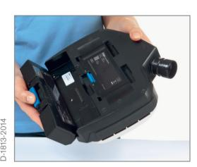
Insert the battery (blue locking button pointing upwards, contacts pointing to the device) into the battery compartment and press until it audibly clicks into place.
