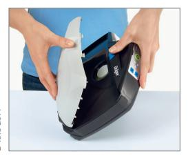
Remove the splash guard from the unit by pressing the blue filter locking button.
