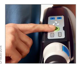
Press the green button on the control panel. The device performs a self-test.
