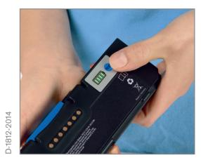
Press the blue button on the battery to show the charging status (indicated by the green flashing LED display).
