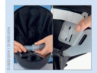
Adjust the head circumference with the support ring. Attach the support ring to the buttons of the head harness so that it rests above the ears.
