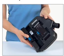
To check the charging status of the battery, remove it from the device by pressing down the blue locking button.
